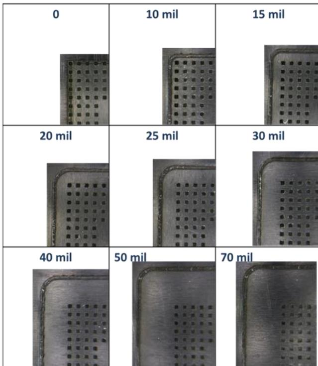
Figure 3a. Welded stencil steps
