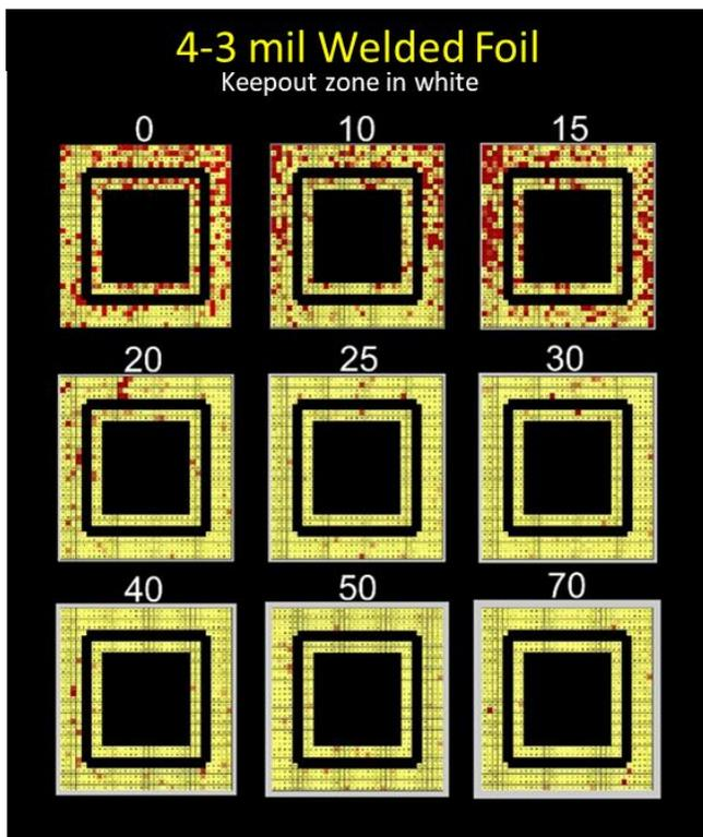
The print-to-print variability is unacceptable up through the 20 mil keepouts on the welded foil, but appears acceptable with the 10 mil keepout on the machined foil.
