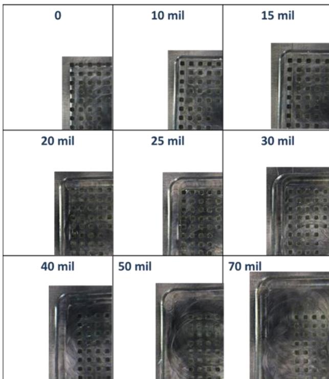
Figure 3b. Machined stencil steps
