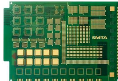
Figure 1. Test PCB
