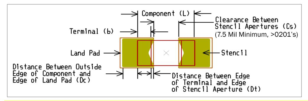
ALWAYS CALCULATE AREA RATIO WHEN CHANGING TO U SHAPE OR INVERTED HOMEPLATE APERTURES
