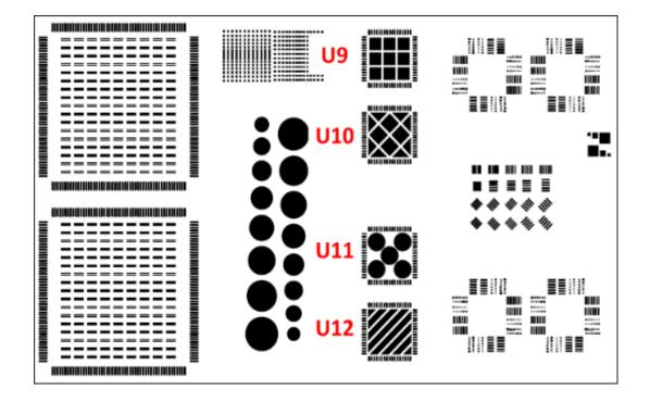
Stencil Design used to determine void percentage based on ground pad stencil design.
