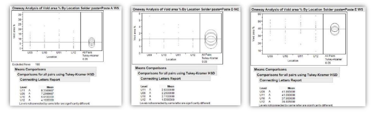
Voiding by stencil design (location) was statistically similar for each of these solder pastes. Stencil design made no difference in this test
