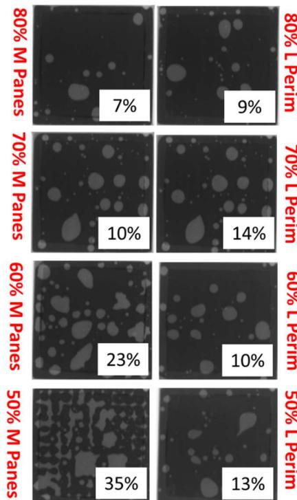
Figure 13. Representative Void Images for the QFN10 Components for the Most Panes and Largest Perimeter Stencil Designs.
