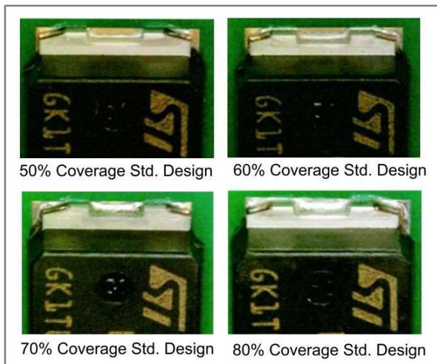
**Figure 6.** Comparison of D-pak Thermal Pad Coverage after Reflow.
