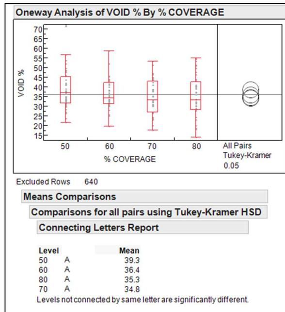
Figure 11. Voiding by Coverage for the QFP144 Component.
