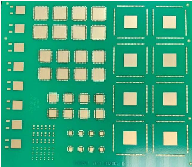
**Figure 2.** Thermal Pad Test Board.
