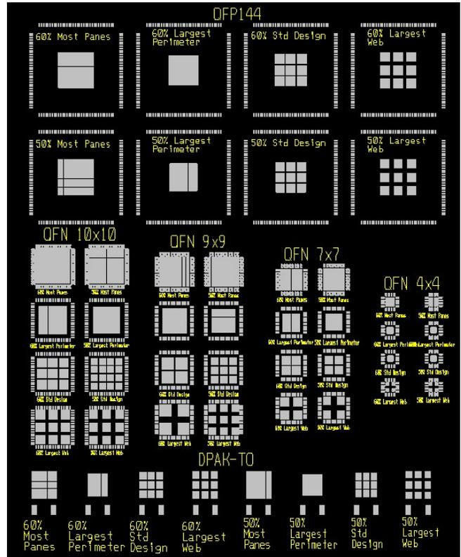
**Figure 4.** Stencil #2 for the Thermal Pad Test Board Which Includes 50 and 60% Area of Coverage.
