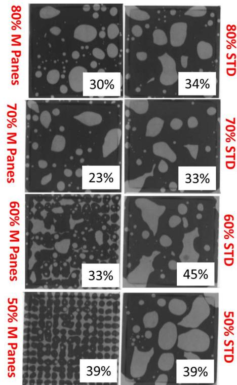
**Figure 15.** Representative Void Images for the QFP144 Components for the Most Panes and Standard Stencil Designs.
