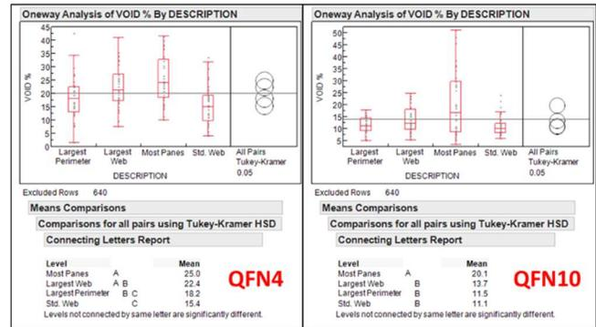
Figure 12. Voiding by Description for QFN4 (Left) and QFN10 (Right).
