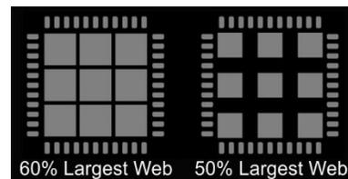
**Figure 1.** Example of a Window Pane Aperture Design on a Bottom Terminated Component Thermal Pad.
