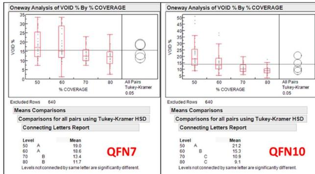
Figure 10. Voiding by Coverage for QFN7 (Left) and QFN10 (Right).
