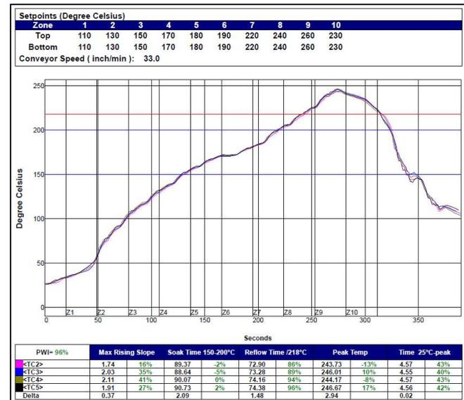
**Figure 5.** Linear Ramp-to-Spike Reflow Profile.
