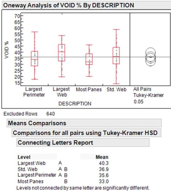
**Figure 14.** Voiding by Description for the QFP144 Component.
