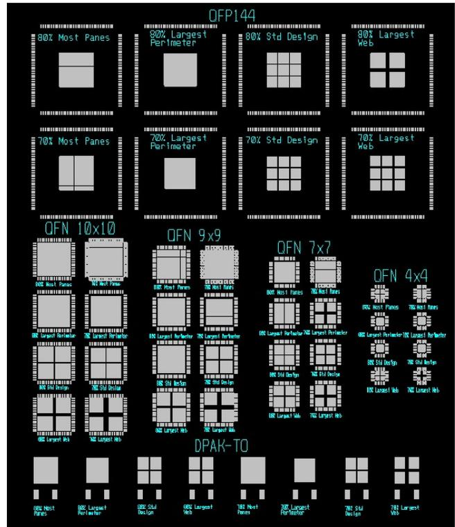
**Figure 3.** Stencil #1 for the Thermal Pad Test Board Which Includes 70 and 80% Area of Coverage.
