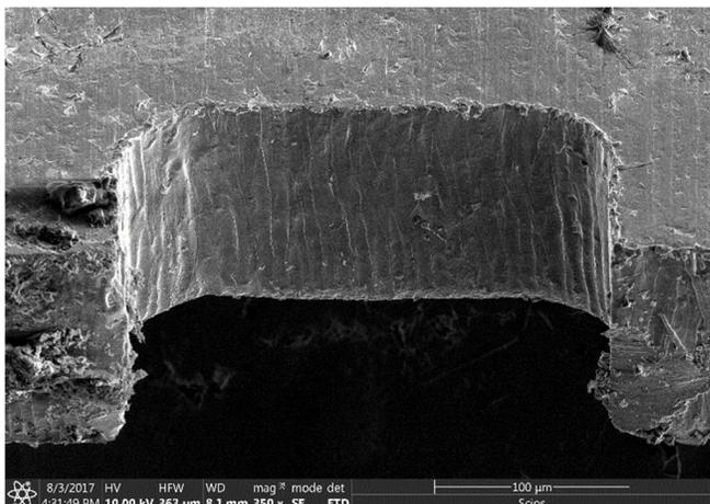
**Figure 17:** SEM of Uncoated Aperture Sidewall, Material 2
