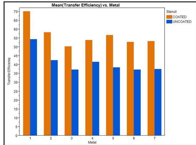
**Figure 10:** Transfer Efficiency for Coated and Uncoated Stencils for All Metals with 0.3, 0.4, and 0.5 Area Ratios combined.
