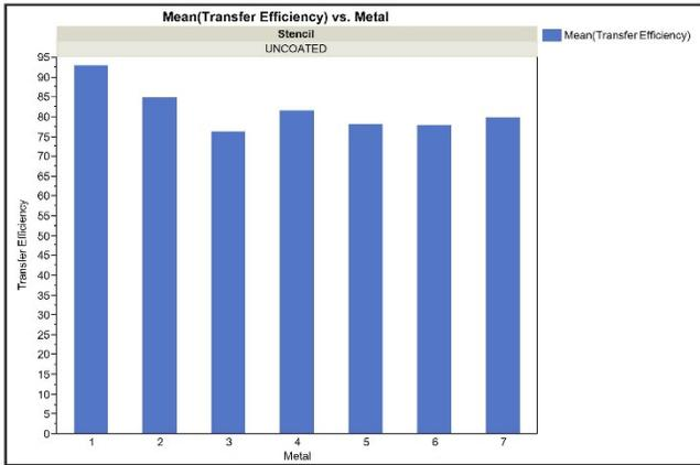
**Figure 5:** Transfer Efficiency of Uncoated Stencils: All area ratios and metal types.
