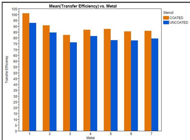
**Figure 9:** Transfer Efficiency for Coated and Uncoated Stencils for All Metals and All Area Ratios.
