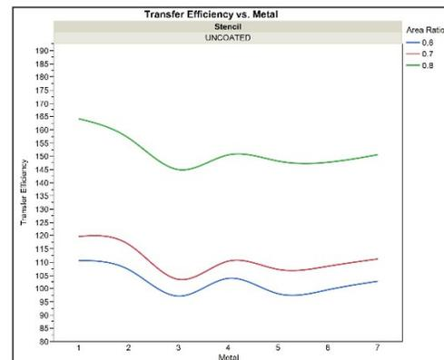
**Figure 8:** Transfer Efficiency of Uncoated Stencils: All metals, 0.6, 0.7, and 0.8 area ratios.
