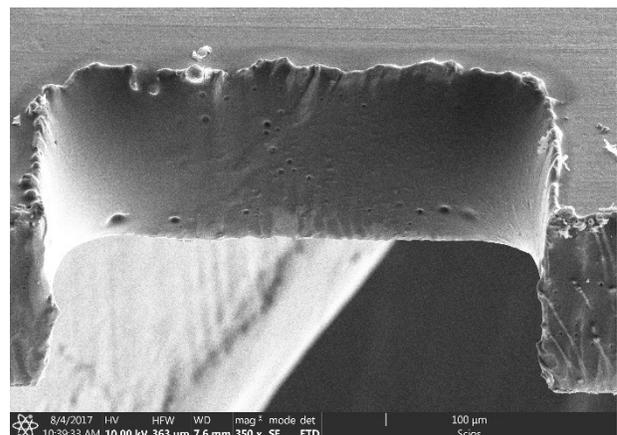
**Figure 20:** SEM of Ceramic Nano-Coated Aperture Wall
