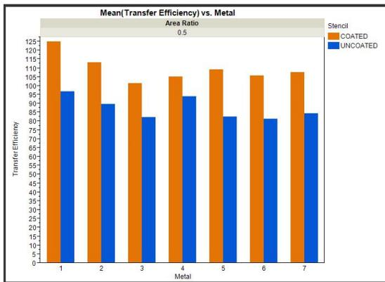
**Figure 11:** Transfer Efficiency of Coated and Uncoated Stencils for all metals and for Area Ratio of 0.5.
