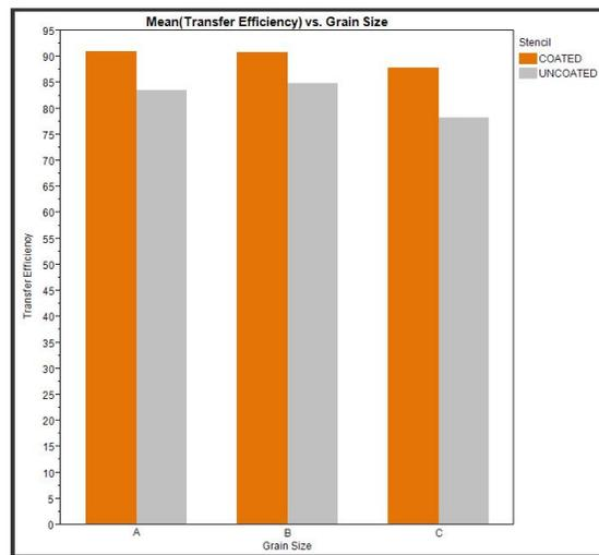
**Figure 13:** Transfer Efficiency vs Grain Size for all Area Ratios.
