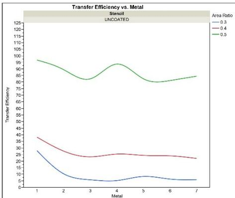
**Figure 6:** Transfer Efficiency of Uncoated Stencils: All metals, 0.3, 0.4 and 0.5 area ratios.
