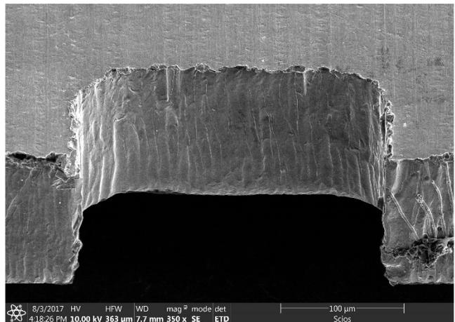
**Figure 16:** SEM of Uncoated Aperture Sidewall, Material 1
