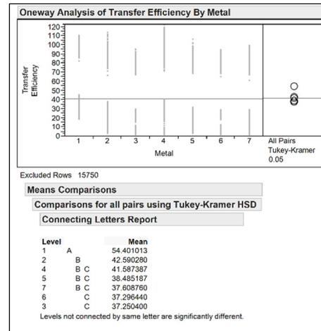
**Figure 7:** Tukey-Kramer HSD on Transfer Efficiency for Area Ratio 0.3, 0.4 and 0.5.
