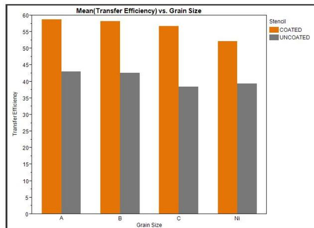
**Figure 14:** Transfer Efficiency by Grain Size for 0.3, 0.4, 0.5 Area Ratios.
