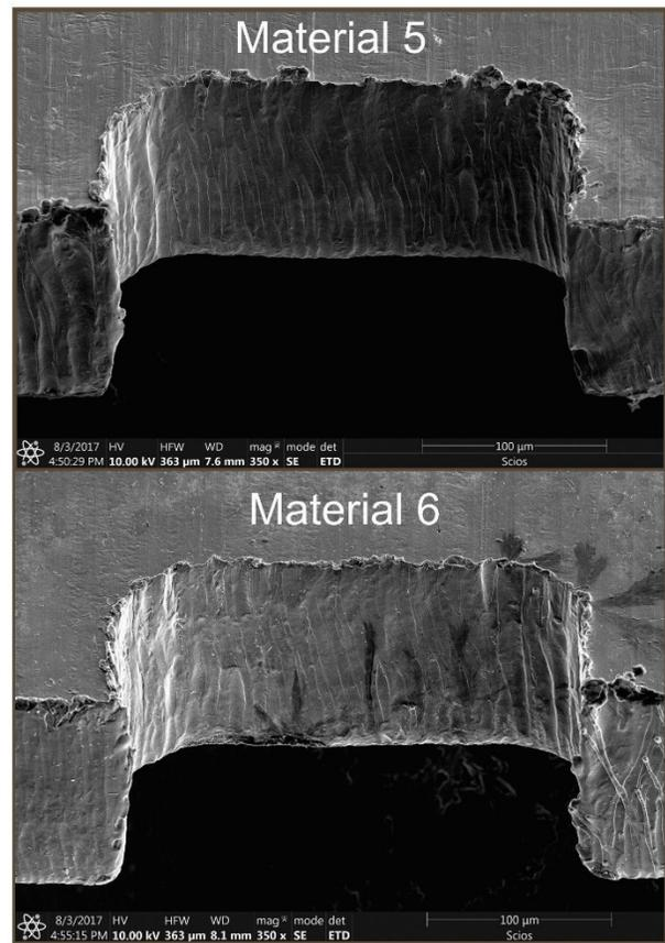
**Figure 19:** SEM of Uncoated Aperture Sidewall, Material 5 and 6
