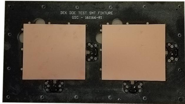
Figure 4: SMT Carrier Fixture.
