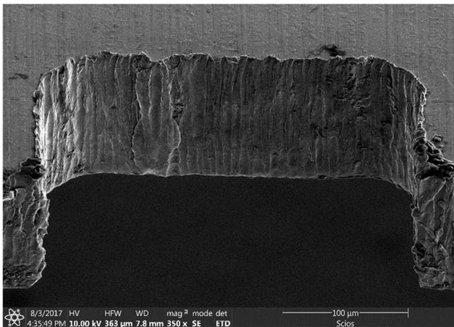
**Figure 18:** SEM of Uncoated Aperture Sidewall, Material 3
